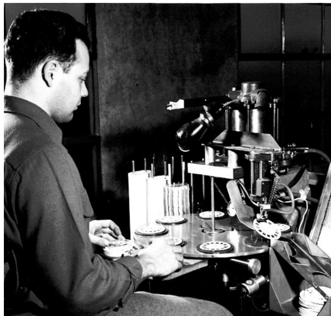
Above: Assembly of the Personal Reel mounts. This process utilizes a special machine developed by Stereocraft.
