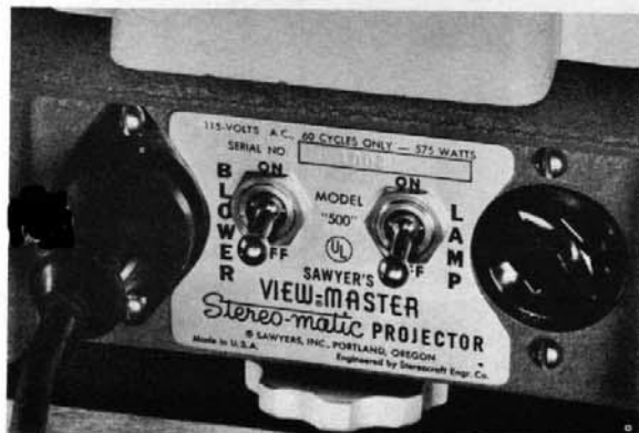
SIMPLE MASTER CONTROL PANEL. Two switches operate all the electrical controls. One switch turns on the blower, the other the lamp. The lamp switch is inactive until the blower is turned on. This prevents over-heating and allows quick cooling after projection show is over.
